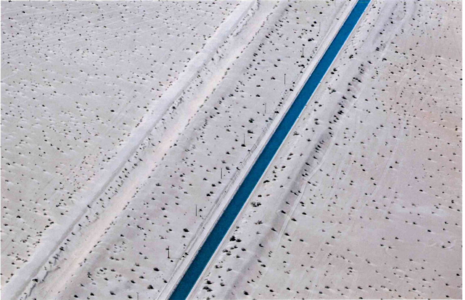
The Coachella Canal is a 123-mile aqueduct that transports Colorado River water from the All-American Canal to the Coachella Valley in Riverside County. (Brian van der Brug / Los Angeles Times)
